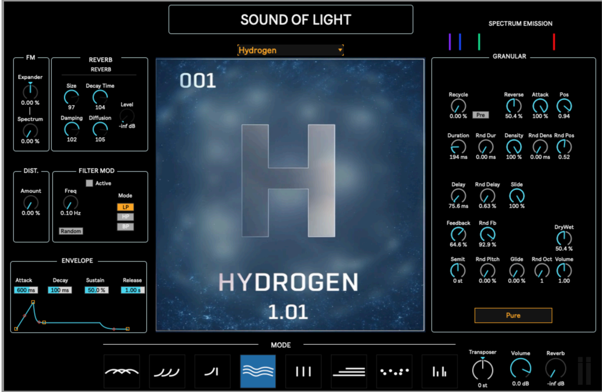
Figure 5: The “Sound of Light” digital instrument interface in Max/MSP, shown with hydrogen selected. Left panel: synthesis and effects parameters; center: element display; right: granular synthesis controls and spectral emission indicator.
